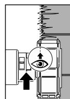
In order to be able to better view the lawn- / curb edge, markings are attached to the safety guard on the right and left, which mark the position of the disc.
