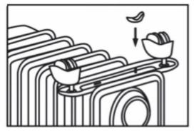
6 Turn the radiator in upright position after the Castor Wheel Assembly fitted.
